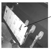
TEMPORARY INSTALLATION OF PASSENGER SIDE SUNVISOR TO ACHIEVE PROPER ALIGNMENT AND POSITION
