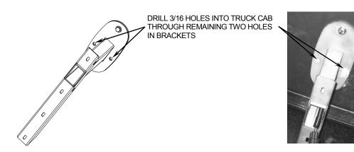
9. Remove brackets from roof and apply a generous amount of supplied silicone into and around all bracket-mounting holes.
